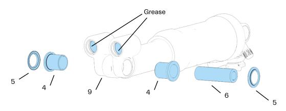
Apply grease to the two bushings inside the slider unit (9). Place the shock in the slider housing unit and press in the two shock bushings (4). Push the shock pin (6) through the bushings and place the slider spacers (5) on the pin, outside of the slider housing.
