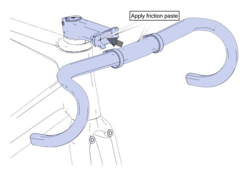
3. Slide handlebar clamps over the protrusions on the side of the stem body. Tighten the four stud screws alternatingly and evenly to 5 Nm. Make sure the gap between the handlebar clamp and the stem body is even. For initial installation, the bolts are coated in thread locker, but if you do adjustments later, use Loctite 243 to secure the bolts. Check the tightness of these bolts before every ride.
